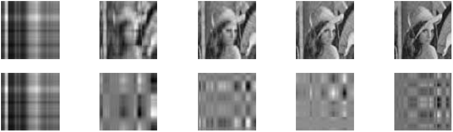
Fig. 2. Lenna reconstructions and components: Top row: Reconstructions using 1, 5, 10, 15 and 20 components. Bottom row: The SVD component images u_i v_i^T corresponding to the first five components.
